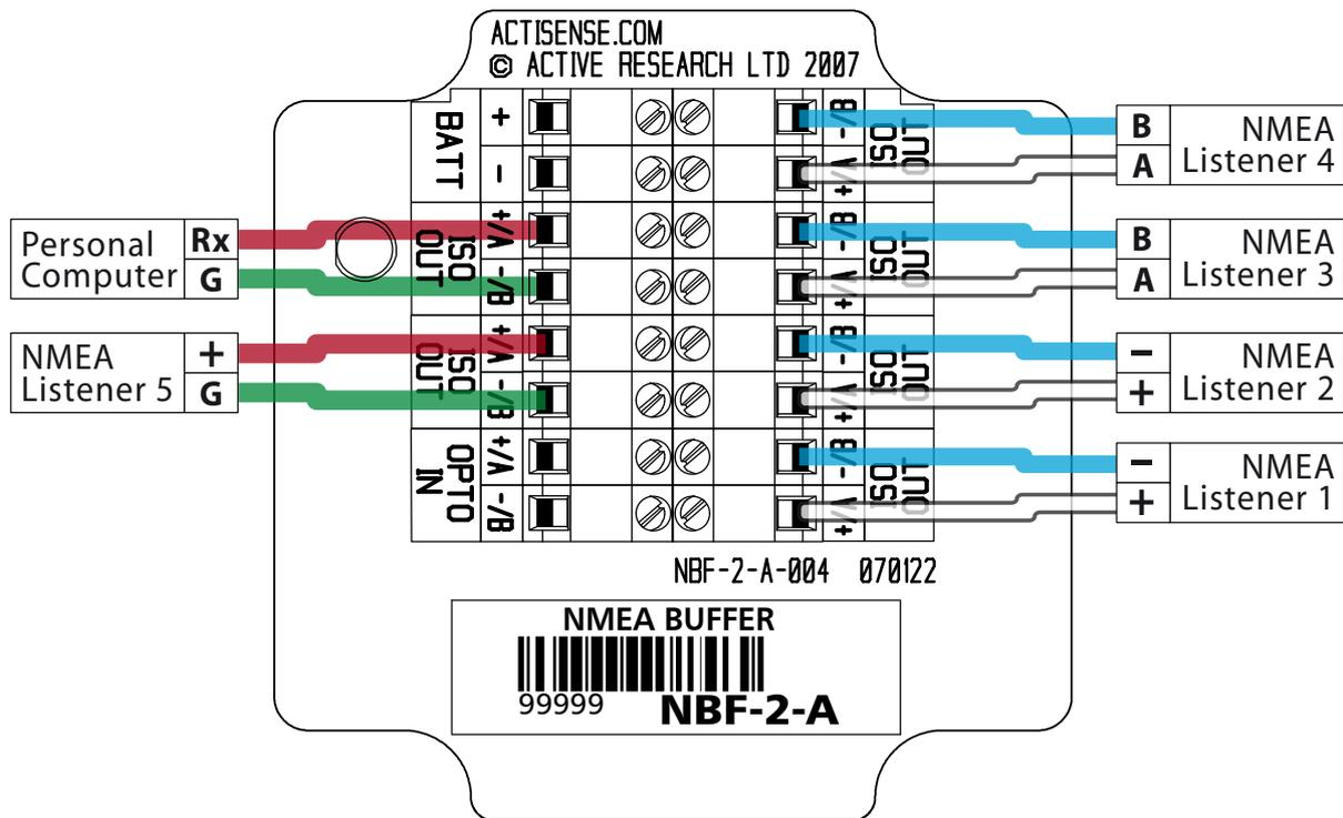
Figure 3 – Output connections
